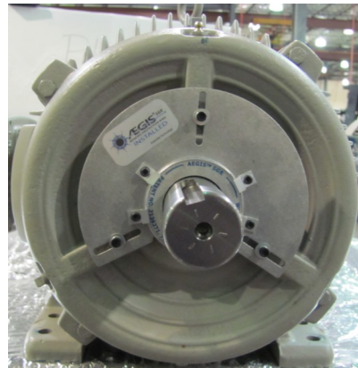
Shaft grounding system installation.
