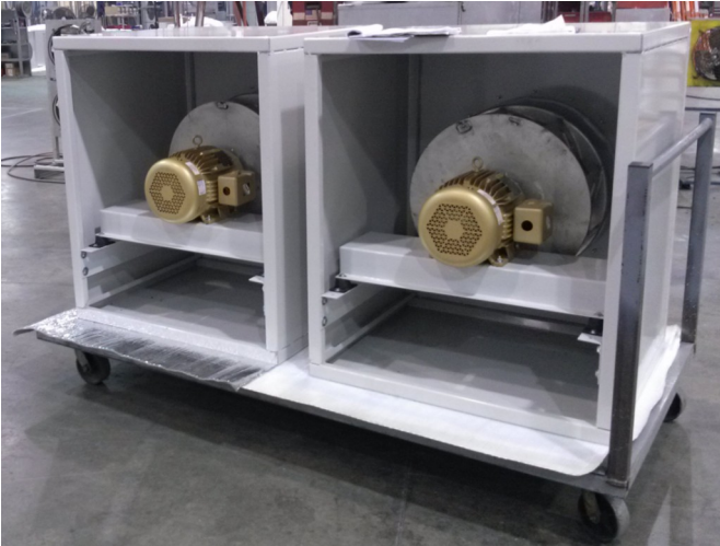
Fan cells can be transported without heavy lifting equipment.
