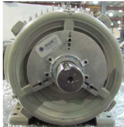
Shaft grounding system installation.
