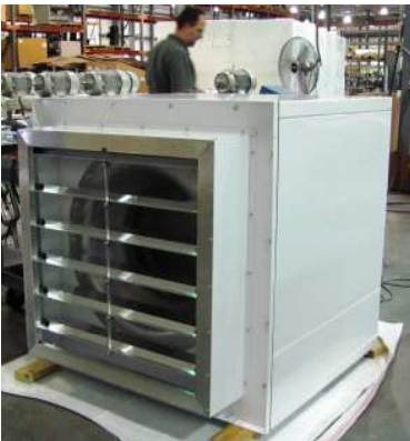
Backdraft damper installation.
