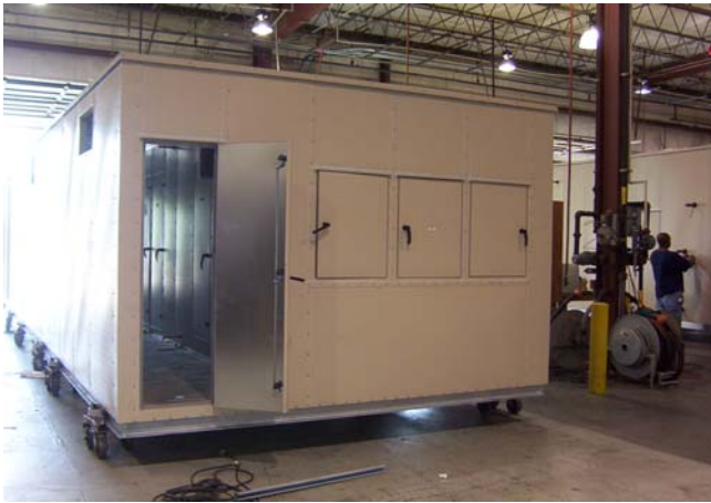
Painted aluminum exterior panels and expanded aluminum condenser coil guards.
