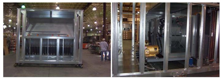
The new direct replacement double deck multi-zone unit with 5 zones will match the roof curb, zones, water, and power connections of the existing unit. Twin plenum airfoil supply and return air blowers with premium efficiency motors, VFD'S, and service lights are some of the features provided.
