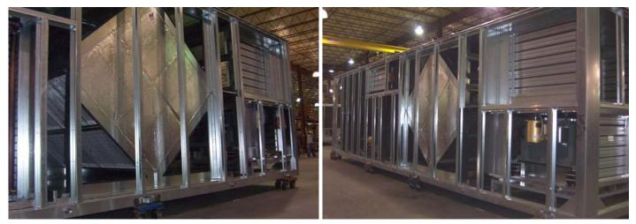
The best alternative was determined to be a plate-type heat exchanger with no pumps, no valves, no water, no moving parts, and the unit efficiency has improved by 25 to 30%. The unit also includes hot water pre-heat and reheat coils.
