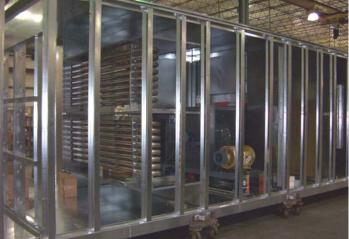
An air cooled condensing section with a total of five (5) independently circuited scroll compressors conditions 14,330 cfm of air down to 41 deg dew point with no need for a defrost cycle. Some other features are plenum supply air blower, premium efficiency motors, VFDS and modulating tubular Heatco burners with stainless steel heat exchangers.
