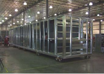
The unit is a top return, top discharge Dual Path VAV system. The fresh air is conditioned with three (3) scroll compressors (lead is a modulating digital scroll) down to 41 deg F dew point. The return air is conditioned thru a separate path with two scroll compressors down to 41 deg F dew point. Each path is provided with an independent subcooling reheat coil and a combined hot gas reheat coil to bring the supply air to 60 deg DB and 50 deg WB.
