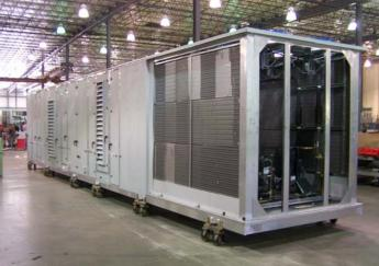
Per the customer's request all access doors are provided on one side of the unit. The unit is completely tested and shipped to the job site for rigging and start up.
