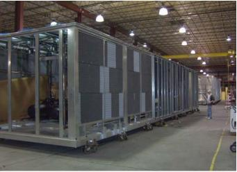
Variable frequency drives on supply and return air blower motors, MERV 13 filters, mist eliminators, Automated Logic DDC controls with BacNet, LonWorks, ModBus and N2 protocol capabilities are some of the features provided with the unit.
