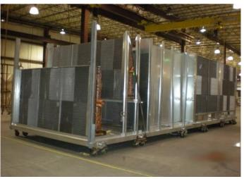
The unit is built in two sections for shipping purposes but it is designed so all refrigeration circuits are intact when the unit is split. The unit has plenum supply and return air blowers with premium efficiency motors and air flow measuring stations.
