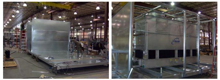
Each unit is 70 feet long. They must be built in sections for shipping but they have been designed so all refrigeration piping will be in-tact when the units ship. 5" insulation on the flooring and evaporative condensing sections are some of the requirements.
