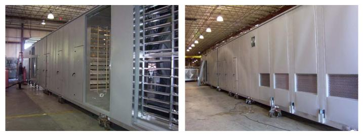
The units are provided with Kynar painted exterior panels and single door handles. The sections are bolted together, completely tested then split in two sections and shipped to the jobsite.
