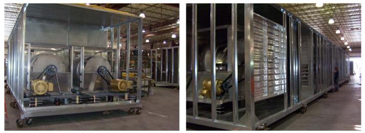
Twin aluminum plenum airfoil supply air blowers and return air blowers with VFDS, outside air airflow monitoring stations, CO2 sensors, high efficiency cartridge filters, and DDC controls are additional features.
