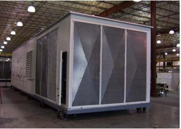
Separate high voltage and low voltage conditioned control panels are required. Kynar painted aluminum exterior panels with single handle, multiple latches doors are additional features. The units are build in two sections to be rigged with a helicopter.
