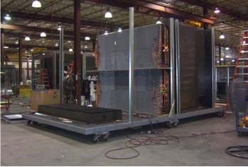
Units consist of formed, welded and coated galvanized steel base, HCFC- free R-410A refrigerant, six (6) scroll compressors piped independently to 6 intertwined DX coils. Isolation dampers and walking grating are provided on supply and return air openings.
