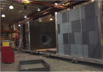
Painted interior liner, 12" cartridge filters, filter rack for future HEPA filters, magnehelic filter gauges with sun shields, photoelectric supply and return smoke detectors and ABB variable frequency drives on supply and exhaust fan motors are some of features provided for the units.
