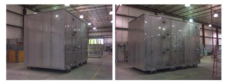
After testing is completed the units are split in two sections, prepared for shipping, and shipped to the jobsite for installation.
