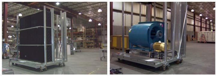
An upblast housed airfoil DWDI blower with TEFC premium efficiency motor and VFD suplies 40,000 cfm of the air through Electro-Fin coated chilled water coils. The cabinet is built in two sections to fit through an opening in the building wall.
