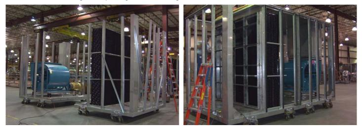
UV lights in chilled water coil section, stainless steel drain pan in all sections, service light in all accessible sections, and 2" pleated plus12" cartridge filters in stainless steel frames are some of the features provided with the units.
