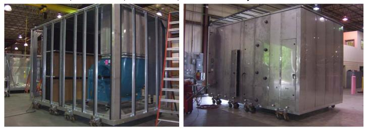
Sections are assembled together to ensure a proper fit, then cased with **stainless steel** exterior and interior panels and tested.
