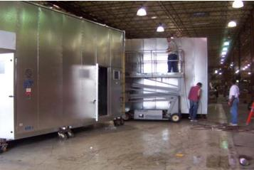
The unit is built in two sections for shipping, assembled together for complete testing and quality control then disassembled and shipped to the job site per the requested onsite date.
