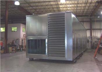
Embossed aluminum exterior panels (never rust), view port windows on all access doors, single door handle with multiple latches and side return air opening are a few other features.
