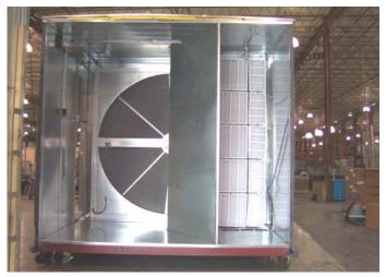
24,000 CFM make up air unit with an Enthalpy Energy Recovery Wheel, 85 tons of DX cooling, 275 KW fin and tube electric heater, Airfoil SWSI plenum supply air are a few options included with this amazing project.
