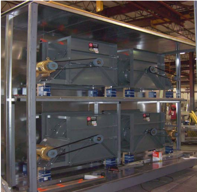
4 airfoil plenum blowers, two 2,000 mbh output propane burners and the unit is built in two sections
