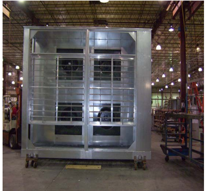
4 airfoil plenum blowers, two 2,000 mbh output propane burners and the unit is built in two sections
