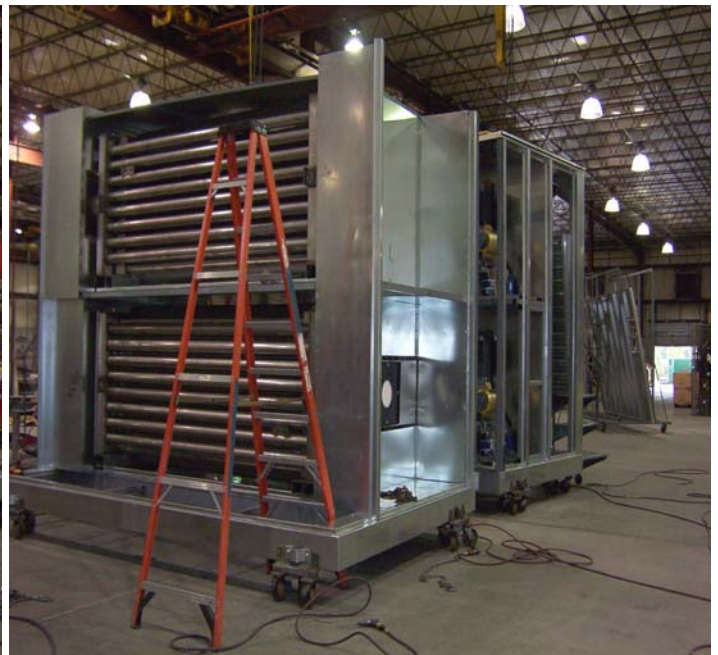
4 airfoil plenum blowers, two 2,000 mbh output propane burners and the unit is built in two sections
