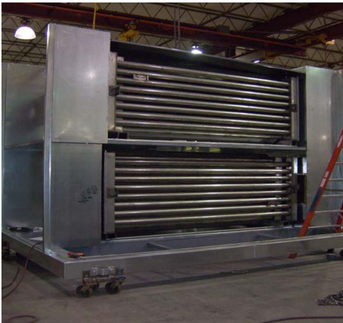
4 airfoil plenum blowers, two 2,000 mbh output propane burners and the unit is built in two sections
