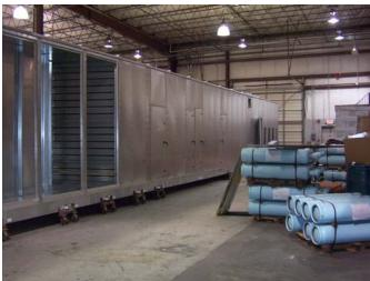
Units are charged with R-134a refrigerant, completely tested and shipped to the job site per customer requested onsite date and time.
