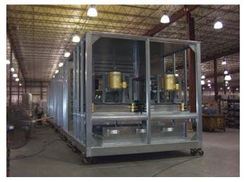
Built in Recold evaporative condensing sections. Twin airfoil plenum SWSI supply and return air blowers with VFDS and isolation dampers. Supply and return air smoke dampers and vapor proof marine lights in all accessible sections.
