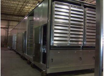
Aluminum exterior panels (never rusts), 2" double wall panels, 5" insulated floor, single door handles with multiple latches,
