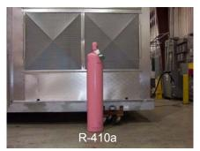
R-410a is the newest girl in town; a blend of R-32 (50%) and R-125 (50%). It is a Replacement for R-22 (not a drop-in), operates at 500 to 600 PSI. Low performance in high- temp. ambient.
