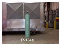
R-134a (tetrafluoroethane, CH2FCF3), one of Replacements for R-22 (not a drop-in), requires 25% to 30% increase in condensing section (coils & compressors) to match R-22.
