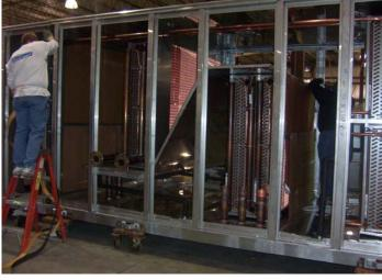
Epoxy-coated airfoil plenum blowers, premium efficiency motors, stainless steel drain pans in every section for wash-down, food-grade caulking, and DDC temperature controls are a few special features.
