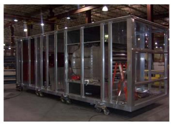
14 row chilled water coils with copper fins and copper tubes and stainless steel casings condition 22,000 CFM of make up air down to 40 deg F dew point. All interior casing and post materials are made of stainless steel. 1,600 MBH input high turn down gas burners with stainless steel heat exchangers.
