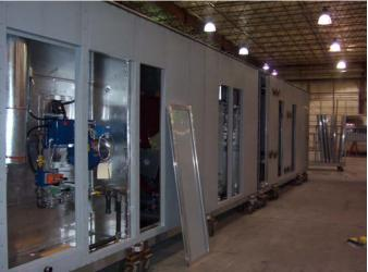
Painted aluminum exterior panels and stainless steel dampers. Doors will open against pressure. The units are built in two sections for rigging purposes, and then assembled together for testing and shipping.
