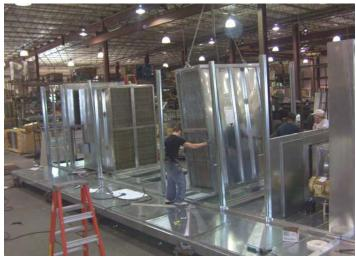
100% outdoor air units with two sets of plate- type air-to-air heat exchangers. The outside air is precooled by both heat exchangers and then re-heated by the second heat exchanger after being conditioned thru the DX coils.
