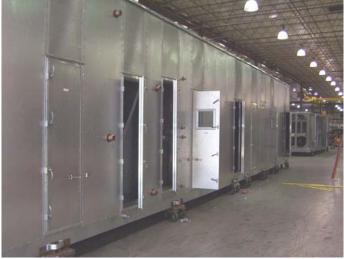
The cabinets are designed for total static pressure of 8.04 (IN-WC), additional liners added to prevent air leaks, then covered with 2" insulated panels with Embossed mill finish aluminum (never rusts) exterior panel.
