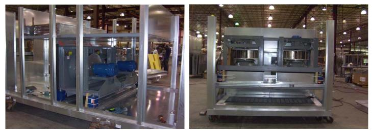
Twin direct drive supply and return air blowers with premium efficiency TEFC motors and VFDS, airflow measuring stations, UV lights, and vapor proof service lights are some of the features provided.
