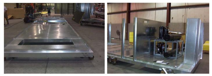
The galvanized steel base and floors are completely welded. The units are provided with conditioned condensing sections with water- cooled shell and tube condensers, digital scroll compressors, and R-410A refrigerant. A water-cooled pre-cooling coil is located in the minimum outside air path to pre-cool the outside air. The coil is piped to the water cooled condensing section.
