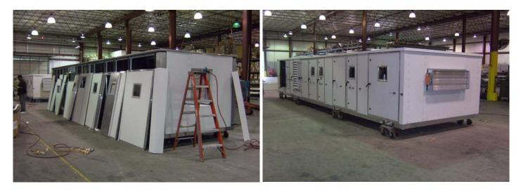
Aluminum Kynar painted exterior panels, 2" foam insulation with R value of 13, hinged access doors with viewports, and single door handles are some of the features.
