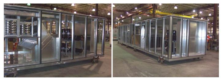
Each unit is provided with multiple Heatco gas burners with stainless steel heat exchangers, high efficiency 12" deep Merv 11 filters, DDC controls, storm proof louvers, individual motor overload protection and disconnect on each motor, and photoelectric supply and return air smoke detectors.
