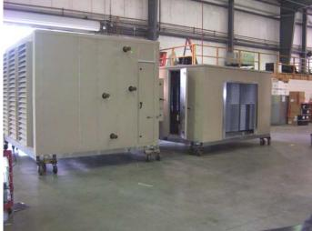
Chilled water and hot water inlet and outlet pipes are stubbed out through the side of the units. The units are tested and prepared for shipping.
