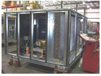
All units are built in two sections (for shipping and rigging purposes), top and bottom sections. Top section consists of an airfoil plenum SWSI blower and hot water coil and the bottom section consists of 12" pleated pre-filters, 12" carbon filters, chilled water coil and the control panel with VFD.
