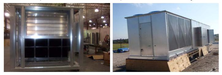
Aluminum exterior panels, hinged access doors with single door handle and multiple latches, 2" pleated pre-filters, 12" deep 95% face loaded final filters, and aluminum airfoil outside air damper are some of the features provided for this unit.
