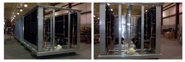
The condensing section consists of three (3) semi-hermetic reciprocating Copeland compressors, Electro Fin coated condenser coils with stainless steel coil casing and compressor support. The condenser fan speed is controlled with VFD for head pressure controls down to 30 deg F ambient.
