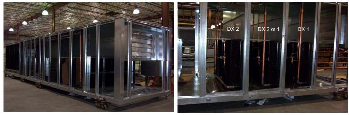
The unit is provided with three (3) equal refrigeration circuits, each circuit is capable of providing 50% of the unit total cooling capacity. One circuit is completely redundant and all circuits are provided with hot gas bypass. The DX coils are Electro Fin coated for seacoast environment.
