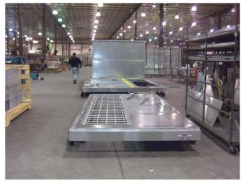
Because the existing unit is shaped like an L, the new replacement unit must be built in two sections for shipping.
