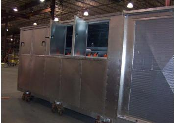
The multi-zone damper is partitioned into 13 zones. Each zone is controlled by a Belimo actuator. The unit has embossed aluminum panels (never rust) and hinged access doors with single door handles.
