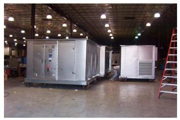
The unit is factory assembled and tested, then split in two sections and shipped to the job site.
