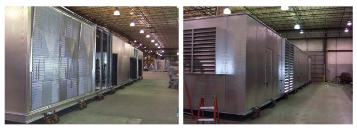
Aluminum exterior panels and louvers are installed, and after completion of testing and quality control, the units are split in two sections again and shipped to the jobsite destination.
