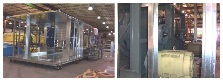
Two Enthalpy Energy Recovery Wheels on both sides of the unit will condition 20,136 CFM of fresh air from 89 degrees F to 80 degrees F. Two SWSI plenum airfoil blowers each with 50 horsepower premium efficiency motor with VFDs will flow a total of 67,120 CFM of air through the unit.
