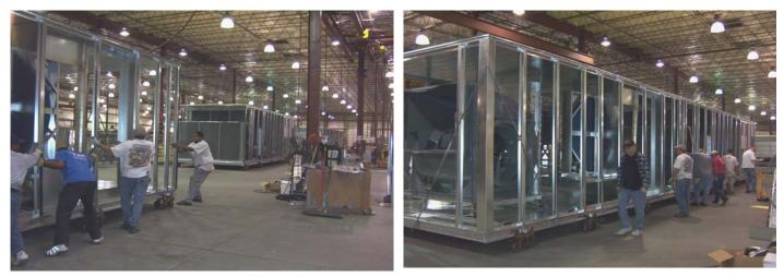
Units are built in two sections each for shipping., After installing all components and assembling the sections together, wiring, and refrigeration piping are completed.
