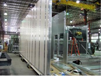
The aluminum exterior and interior panels are insulated with 3 inch polyurethane foam insulation with R value of 20.
