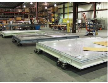
Units are built in sections with structural steel bases, welded aluminum tread plate floors, drains in all sections, removable lifting lugs and 2 inch turned up lip around the base perimeter and floor penetrations.
