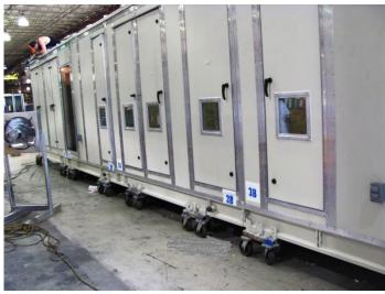
Units are completely assembled, performance and air leak tested.
