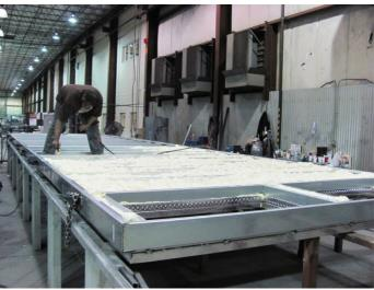
The entire base frames are fully welded and covered with welded aluminum treadplate floors. A 2 inch upturned flange is provided around the base perimeter. The bases are sprayed with 4 inches of polyurethane foam insulation.
