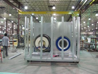
Because of the critical sound levels, Acoustiflo blowers with built in diffusers, direct drive TEFC motors and VFDs have been used on supply and exhaust air fans.
