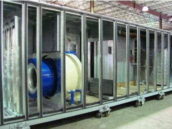
Enthalpy energy recovery wheel, Spiral finned electric heater with SCR controls, aluminum airfoil dampers and piezometer rings are some of features provided.
