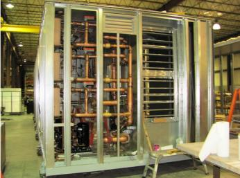
Multiple independent refrigerant circuits are completely piped. Each circuit is provided with an independent hot gas re-heat coil and a brazed plate water cooled condenser.
