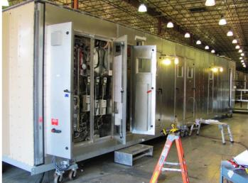
Cabinets are pressure tested for air leaks and units are fully run tested for operational performance by factory technicians before shipping.
