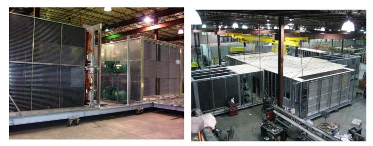
The unit is built in 6 sections for shipping, but it is designed so that all circuits are intact when the unit is shipped.
