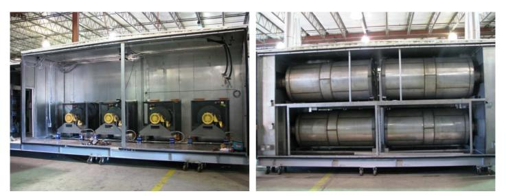
Four (4) direct drive airfoil plenum blowers with VFDs and four (4) Power Burners with drum and tube heat exchangers are additional features of the unit.
