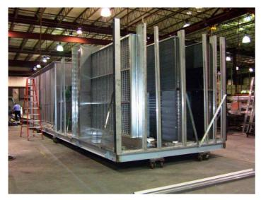
Hot gas reheat coil, sub-cool reheat coil, 126 KW electric heat ,
