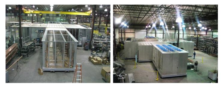
Aluminum exterior panels are insulated with 2" polyurethane foam insulation. The unit is completely tested and shipped to the jobsite.
