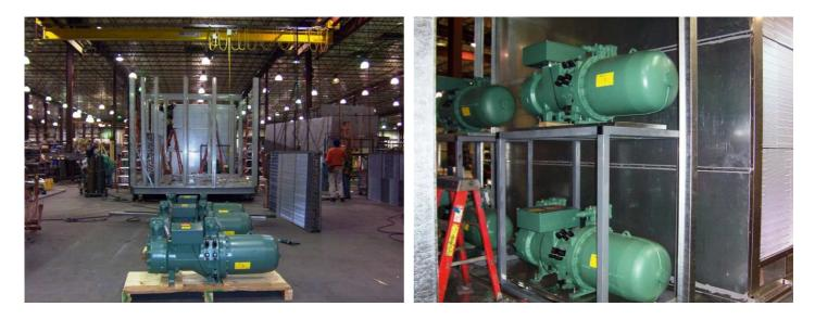
The unit consists of two air cooled condensing sections with eight (8) eighty ton screw compressors.
