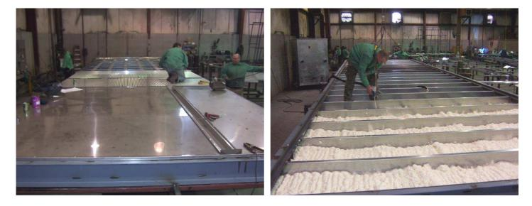
The base is constructed with 8 inch welded structural steel and it is sprayed with 4 inches of polyurethane foam insulation.
