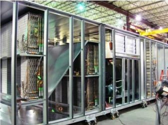
The two 149 tons units are built in two sections each for shipping and rigging. They are designed so that all refrigeration circuits are intact when the units are shipped and placed into operation. No field piping is required.
