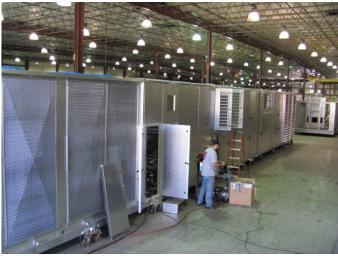
Units are cased with 2" polyurethane foam injected aluminum panels, tested, split in two sections and shipped to the jobsite.
