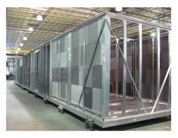
Twin airfoil plenum SWSI blowers with premium efficiency TEFC motors with Heatco tubular type burners are some of the features provided in the units.
