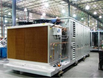
The unit is cased with 2" aluminum polyurethane foam insulated panels, charged with R-134a refrigerant, completely tested and shipped to the job site.
