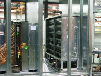
100% make-up air unit with DX cooling, integral face and bypass (IFB) hot water coil build to cool and heat the space to the design conditions.
