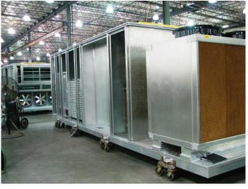
Muller water cooled / air cooled condenser with evaporative cooling pads, microchannel heat exchanger and Ziehi-Abegg Owlet AC & EC fan systems, lowers power consumption, lowers operating costs with no water treatment chemicals required.
