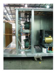
Wrap around heat-pipes, screw compressors, plenum airfoil SWSI blower with premium efficiency motor and a VFD are some of the features provided.
