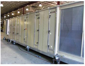
The unit is cased with Kynar coated aluminum exterior panels and insulated with 2" polyurethane foam insulation. The united is completely tested and shipped to its destination.
