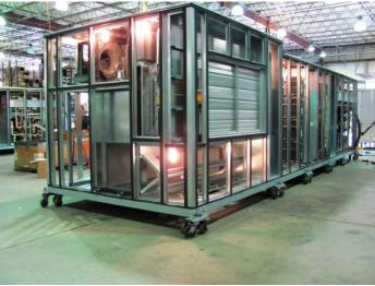
Service lights in all accessible sections, perforated liners in blower sections, and doors that open against pressure with internal door handles are additional features provided.
