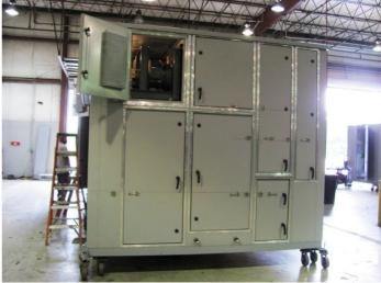
The exterior panels are Kynar painted galvanized steel, insulated with 2" foam polyurethane. The doors are mounted in welded extruded aluminum frames. The units are tested and shipped to the jobsite.
