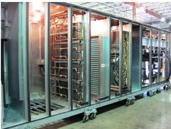
Each refrigerant circuit is piped independently and has a dedicated hot gas reheat coil for humidity control.
