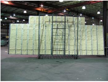
The entire base frames and roof structures are fully welded and sprayed with polyurethane foam insulation. Base frame is painted with epoxy primer.
