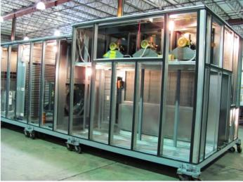
Some of the features provided include two stage energy recovery systems utilizing flat heat pipes and aluminum air-to-air plate heat exchangers and direct drive air foil plenum supply air and exhaust air blowers with VFDS.
