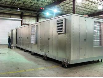
The units are cased with 2" aluminum polyurethane foam insulated panels, tested and shipped to the jobsite..
