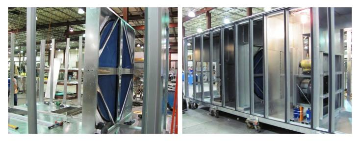
Six (6) of the units are packaged water cooled heat-pump systems with energy wheels, digital scroll compressors, R-410a refrigerant, plenum supply and exhaust air blowers with VFDs, air flow measuring stations and wire resistance electric heaters.
