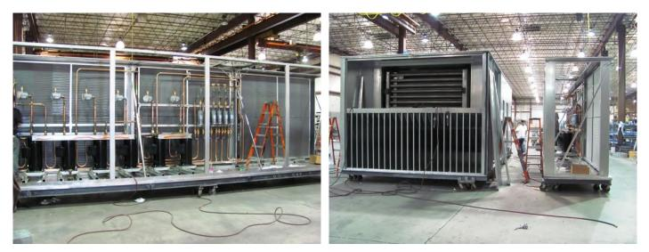
Six (6) scroll compressors, two (2) airfoil SWSI plenum blowers with premium efficiency motors and return air blowers are some of the features provided. Unit is built in two sections for shipping.
