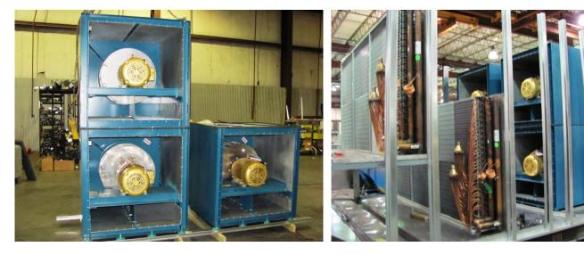
The supply air blower section consists of four (4) modular direct-drive plenum fans, stacked in an array with acoustically-lined internal walls.
