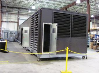
The units are cased with 2" double-wall foam insulated panels, with Kynar painted aluminum exterior and galvanized interior, completely tested and will be shipped to it's destination
