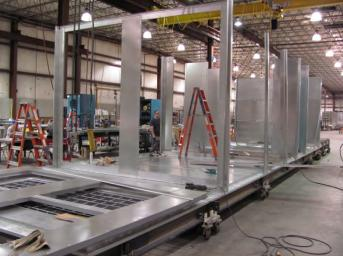
The entire floor of the units are welded and have a 2 inch turned up lip around the base perimeter. All posts are made out of galvanized steel and insulated with foam insulation.
