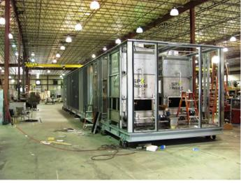
High turn down natural gas power burners, airflow measuring stations, CO2 sensors, access door view ports, vestibule exhaust fan, vestibule electric heaters and condensate water recycling system are some of the features provided.
