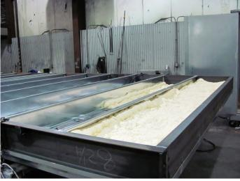
The unit base frames are built with welded structural steel, welded cross rails and channels, and sprayed with 6 inches of polyurethane foam insulation.
